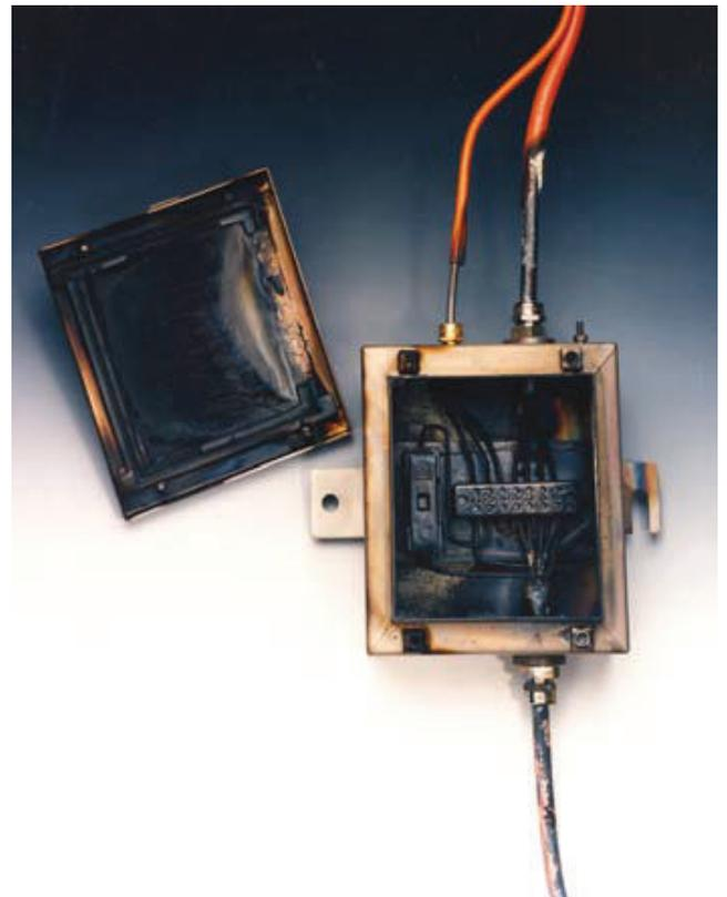
On the successful conclusion of this test, which is designated "fire-alone" BS6387'C', the next test is to mount the sample (still powered-up) on a flat vertical surface and to apply flame at a temperature of 950°C (1742°F) (by means of a flame gun) whilst at the same time striking the board on which the sample is mounted with a 25mm (1") diameter iron bar every 30 seconds for a period of 15 minutes. This is designated the "impact test" BS6387 'Z'.
