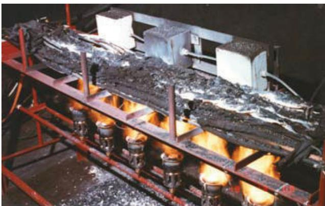
After the test it was found that the body of the nylon terminals had disappeared completely, the melamine body had taken on the appearance of biscuit (because the wood filling had burnt away) and only the ceramic bodied terminal appeared to be intact.
